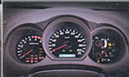
2. Illuminating Optitron gauges offer brightness adjustability and better readability.
