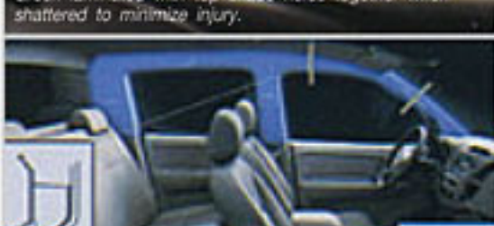
Shock-absorbing door structure to reduce injury in case of accident.
